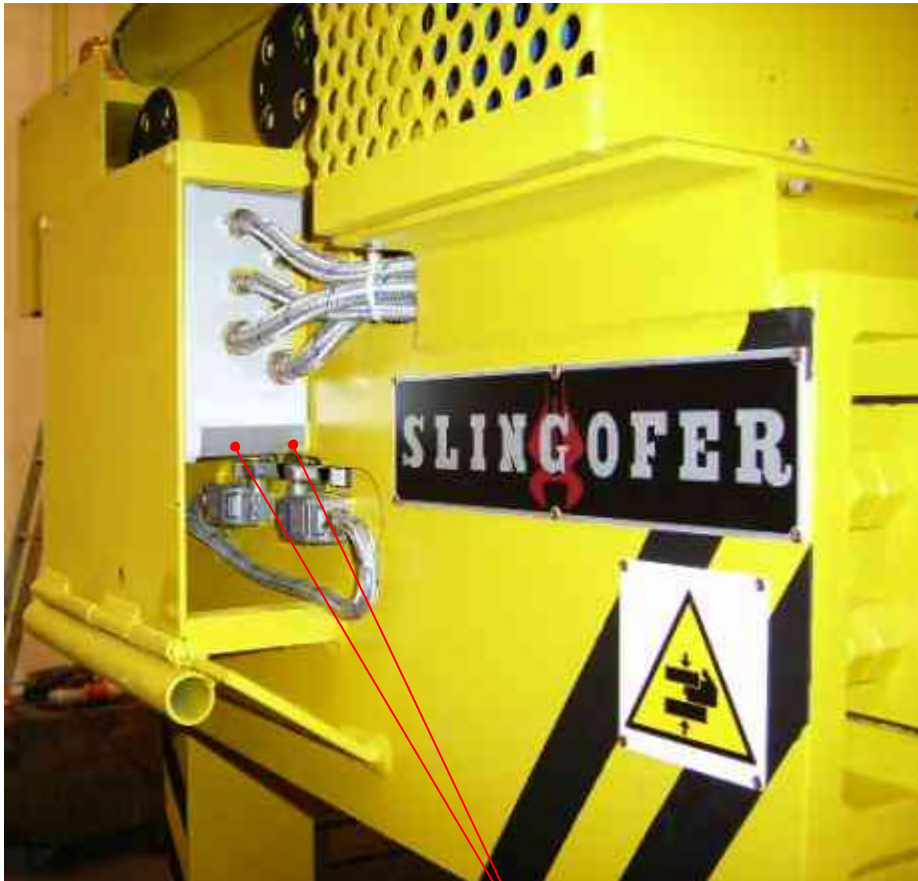
MAX. AND MIN. OPENING LIMIT SWITCHES
