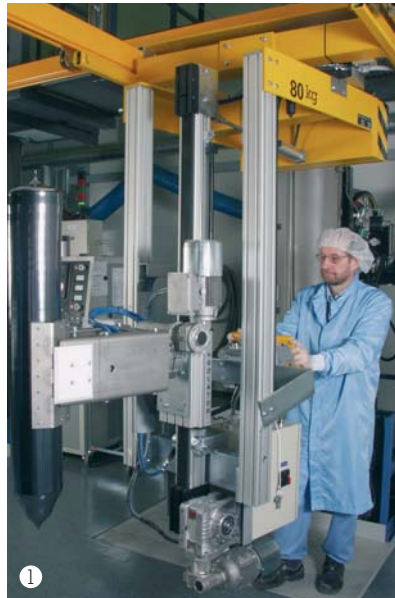
Special solution: using ERGOLATOR® to lift silicon ingot from an oven, turning it and placing the ingot on a transportation cart.
