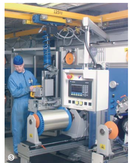
Lifting of a light cable roll from a rack with an ERGOLATOR® and placing the roll into a machine.
