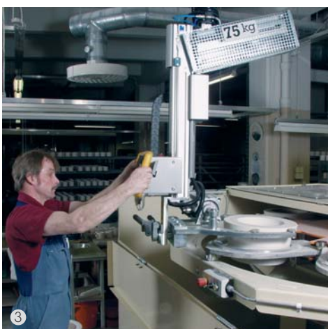
Lifting of a casting model with ERGOLATOR® from a pallet and placing into a machine.
