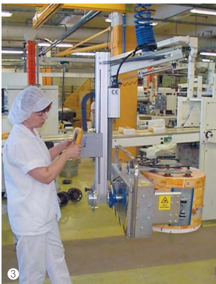
Handling of big rolls by gripping the roll from outside to leave the centre hole free.
