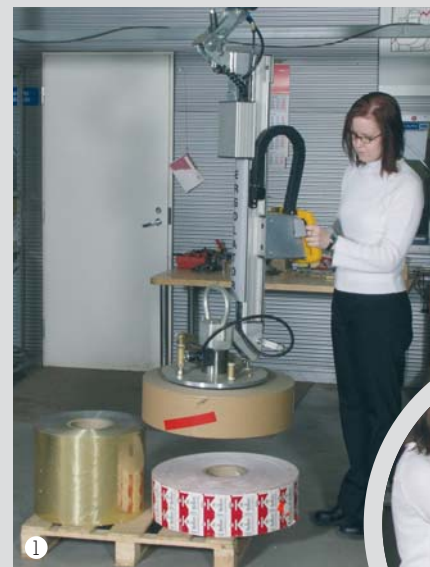
Lifting rolls with a big suction pad from/to pallet in a horizontal or vertical position.
